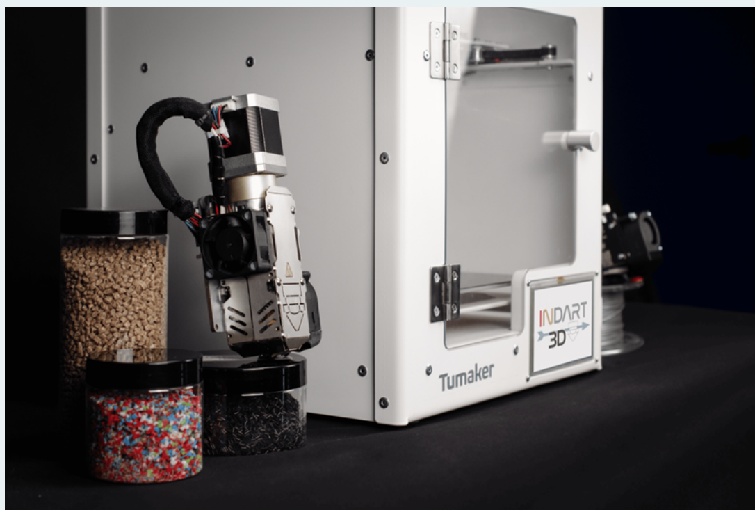
Figure: Tumaker modular 3D printer with pellet extrusion system. The setup highlights its versatility, commitment to sustainability, and potential for research into new pellet-based materials.
