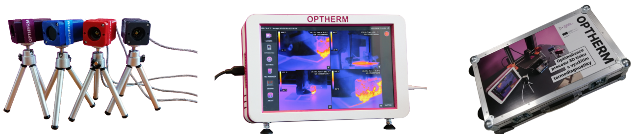
Figure: Complex measurement system with software LabIR OPTHERM for IR thermodiagnosics of FLM 3D printing process
